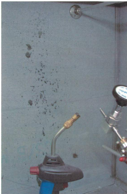
Figure 5: Picture of Tire Lyna which Splattered onto Wall of Lab Hood
